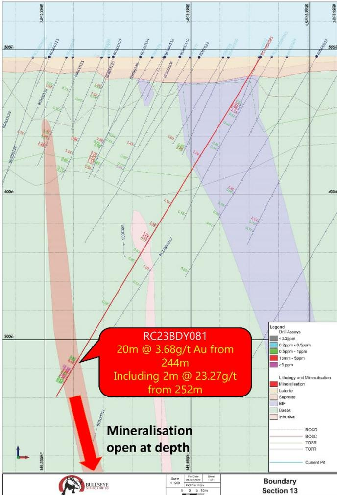
**Figure 21 | Section B Cross section in the Neptune prospect showing wide, high-grade zones of continuous mineralisation which is untested at depth. Black drill traces are historic drilling and Red drill traces is drilling completed during the Quarter**
