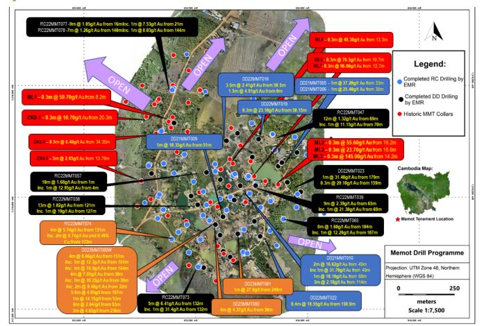
Figure 7 | Memot artisanal workings with recent (orange) previously announced (black and blue) and historic (red) drill collars and significant intersections
