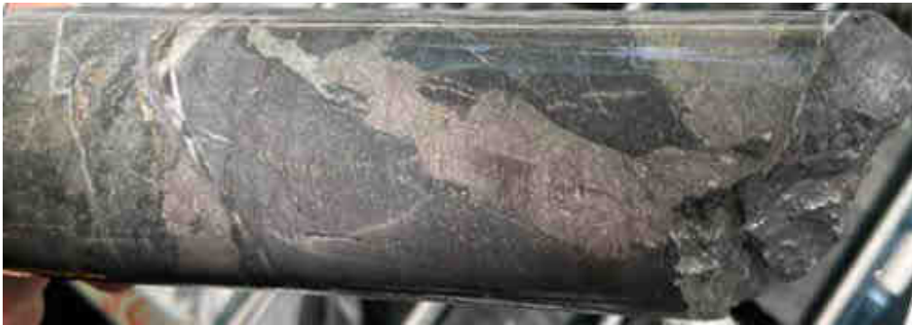
Figure 10 | High grade sulphide (arsenopyrite, pyrrhotite and pyrite) mineralisation from RCDD22OKV444, 6m @ 14.10g/t from 323m
