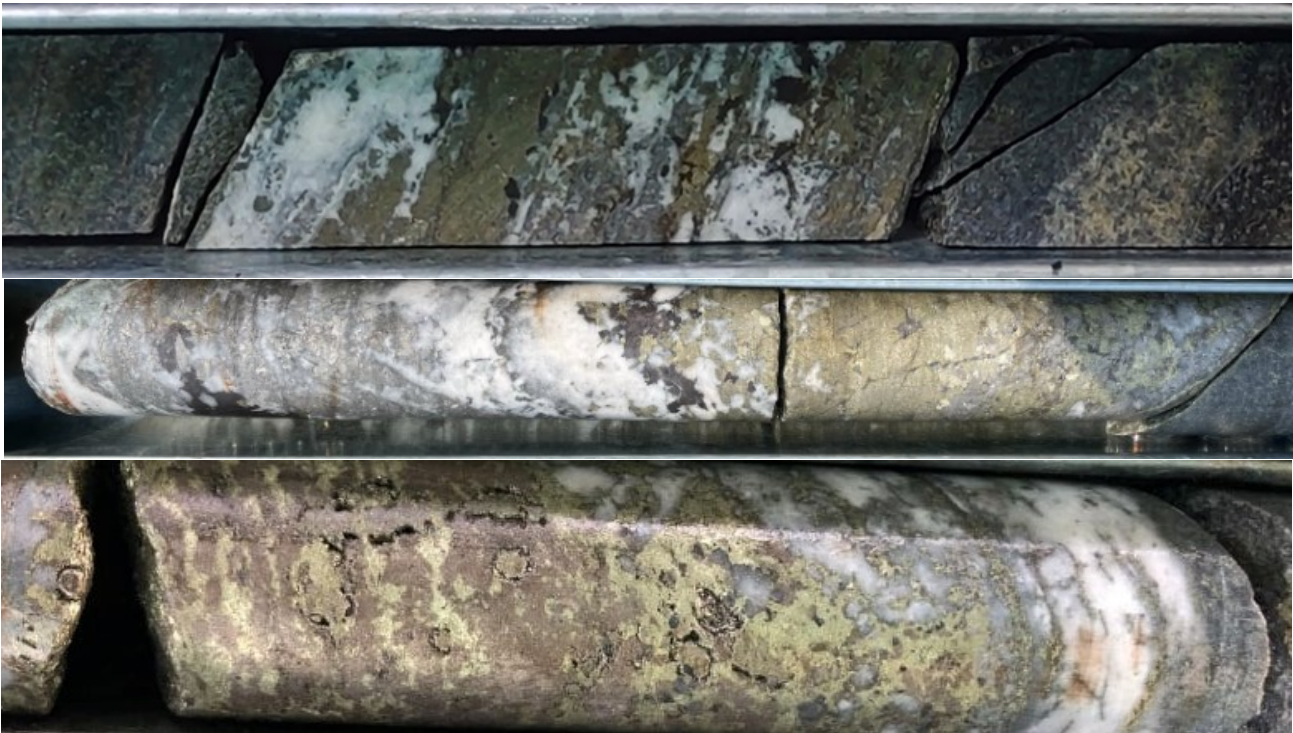
Figure 7 | Mineralised veins in Memot Diamond Core. Quartz veining with Pyrite, Arsenopyrite, Pyrrhotite, Chalcopyrite and Sphalerite sulphides. Top: DD21MMT001 - 1m @ 8.91g/t, 2.16% Cu from 48m Middle: DD22MMT013 - 0.4m @ 17.70 g/t Au, 230 g/t Ag, 2.78% Cu, 0.56% Pb and 1.74% Zn from 190m Bottom: DD21MMT006 – 1m @ 25.4 g/t Au, 73 g/t Ag, 1.81% Cu, 0.1% Zn
