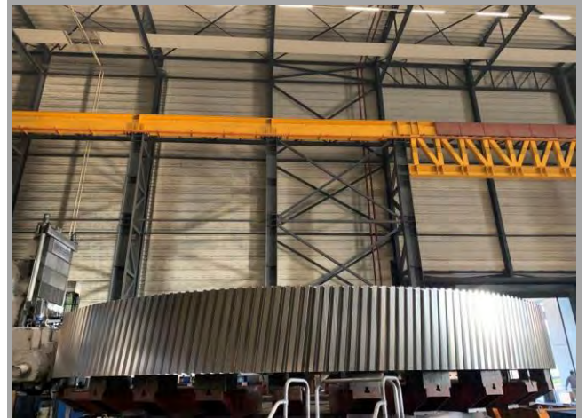
Figure 5 | Mill Girth Gear
