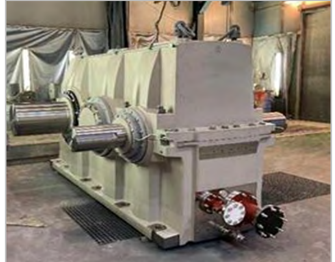
Figure 7 | SAG Mill Gear Box
