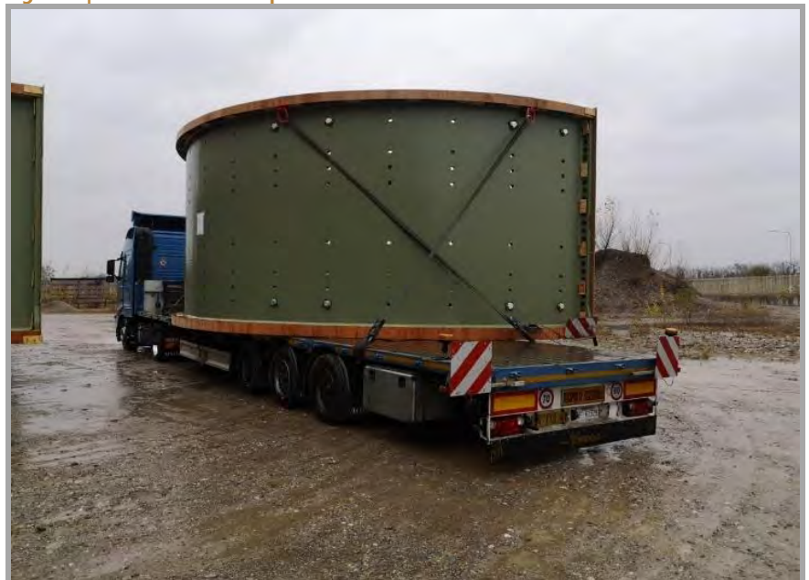
Figure 9 | Mill Shells in Transport
