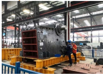
Figure Twenty One | Trial Assembly of Primary Jaw Crusher
