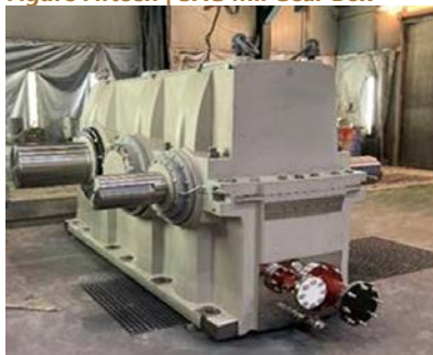
Figure Fifteen | SAG Mill Gear Box
