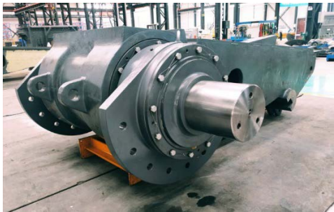
Figure Twenty | Primary Jaw Crusher
