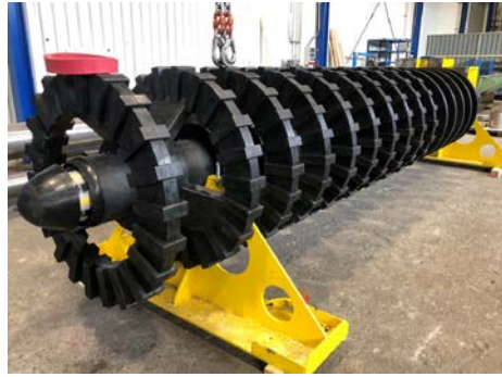
Figure Eighteen | Regrind (HIG) Mill Main Shaft
