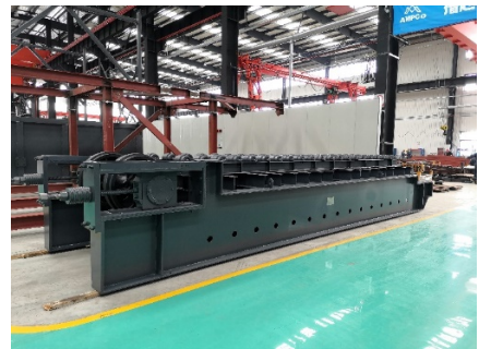
Figure Twenty Five | Apron Feeder
