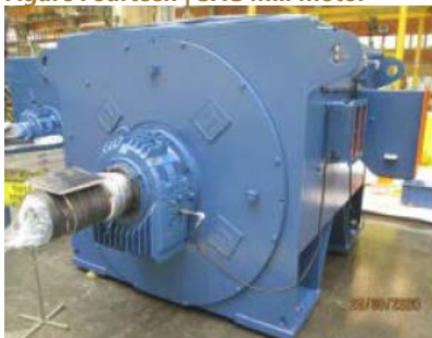
Figure Fourteen | SAG Mill Motor
