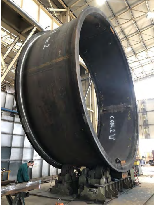
Figure Eighteen | SAG Mill shell
