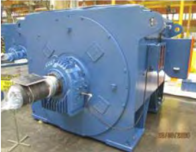
Figure Twenty | SAG Mill motor
