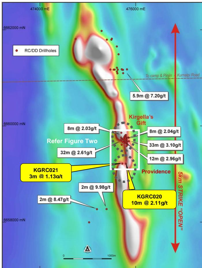
Figure Two | Providence Prospect Anomaly and Drill Hole Collar
